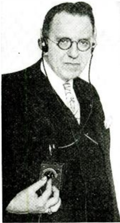
The Vest-Pocket short-wave receiver in operation; a sensitive pair of headphones such as the Trimm 4,800-ohm "featherweights," or the new Brush "crystal" phones will provide a very sensitive receiver.
